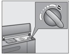
Turn the rotary selector for the grinder counter-clockwise for a finer grind or clockwise for a coarser grind.
